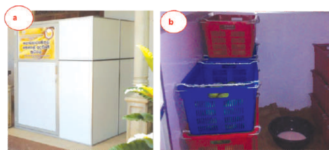
Figure 6. Airtight chamber developed by the National Institute of Postharvest Management (NIPHM), Anuradhapura, for ripening of fruits by ethylene gas (a); mango stacked in plastic crates in the chamber and ethephon solution in a container at the center of the chamber (b)
